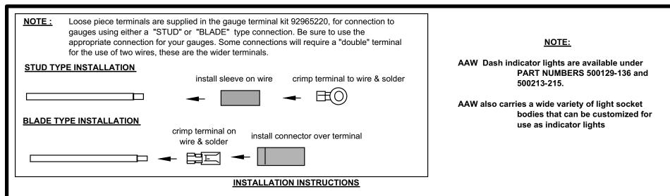
Gauge disconnect connectors are provided for ease of installing and removing the gauge cluster and can be located at a convenient point between the gauge cluster and the under dash harness. A gauge terminal kit, 92965220, is provided for the gauge connections. It is recommended that all ring terminal and blade terminals be soldered. Do not solder the bare wires that are connected to the panel. This connection is made to work with bare stranded wire.
